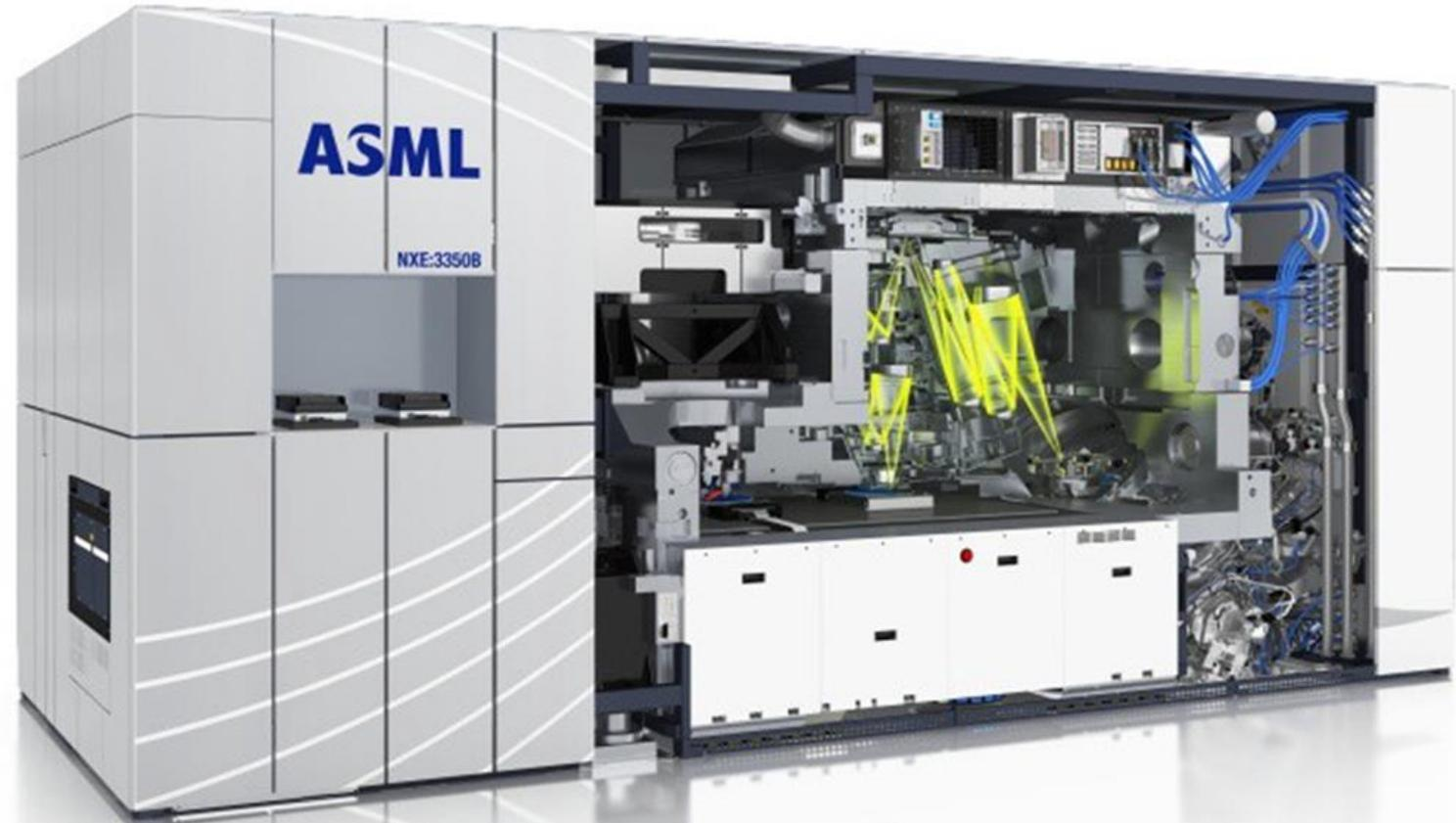
Sources: ASML TWINSKAN NXE: 3350B 13.5-nm EUV projection system.
