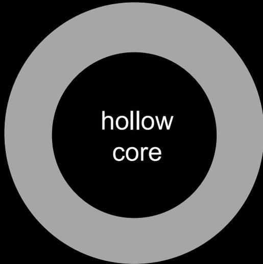
optical modes of hollow waveguides always have anomalous dispersion (geometrical effect)
