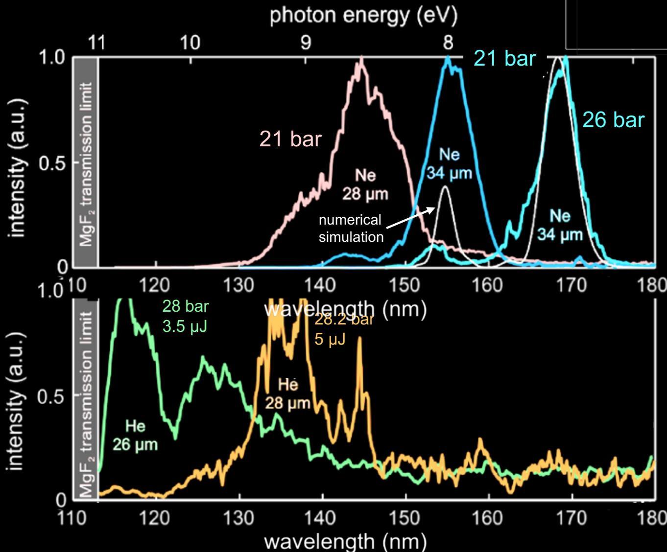
Coherent ultrashort DW pulses of VUV light generated in Ne-filled HC-PCF (35 fs, 4 μJ pump at 800 nm)
