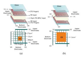
Fig. 1. PS-BPLC beam steering structure. (a) Blazed grating, (b) continuous phase. The orange areas,  $C_1$  and  $C_2$  are the studied regions. Note: drawings are not to scale.
