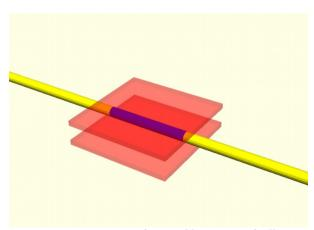
Fig. 1. Fig. 1. Setup of PLCF (blue section of yellow optical fiber) with NP-doped LC response for electric field with various modulation frequencies placed between two plates(red)
