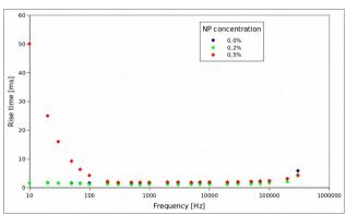
Fig. 4. PLCF rise times induced by external electric field for wide frequencies range for concentrations 0.5% wt. to 0.2% wt. and 0% wt.
