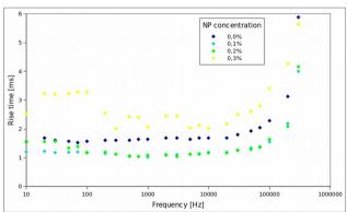
Fig. 5. PLCF rise times induced by external electric field for wide frequencies range for concentrations 0% wt. - 0.3% wt..
