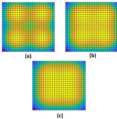
Fig. 8. The 2D view of light distribution for different values of LED emission angle: (a) 30 degrees, (b) 50 degrees, and (c) 70 degrees.
