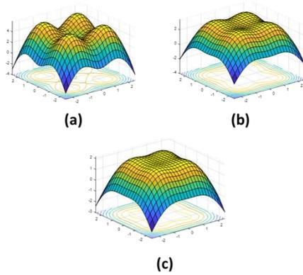
Fig. 7. The 3D view of light distribution for different values of LED emission angle: (a) 30 degrees, (b) 50 degrees, and (c) 70 degrees.
