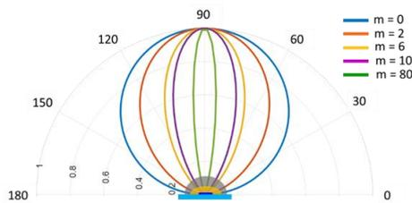
Fig.3. The luminous distribution curve of LED with different values  $m$ .
