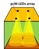
Fig. 5. Illustration of modeling with using 4 LEDs.
