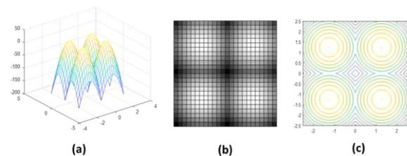
Fig. 6. Uniformity of case using the LEDs with semi-emission angle at half power of 5 degrees. (a) 3D view., (b) 2D of light distribution., (c) contour of light distribution on the floor.
