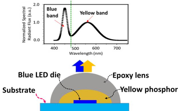
Fig. 1. Illustration of white light generation method (bottom) and its emission spectrum (top).
