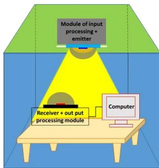
Fig. 2. Illustration for pcW-LEDs based visible light communication principle.
