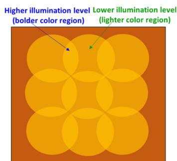
Fig. 4. Illustration of un-uniform light distribution caused by LED light source on the floor.
