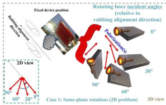
Fig. 4. Core experimental approach in incident angle study (2D view represents resulting laser polarizations rotated in same 2D planes relative to fixed rubbing alignment direction). Measurement results based on setup maintaining laser driving current of 3 A.
