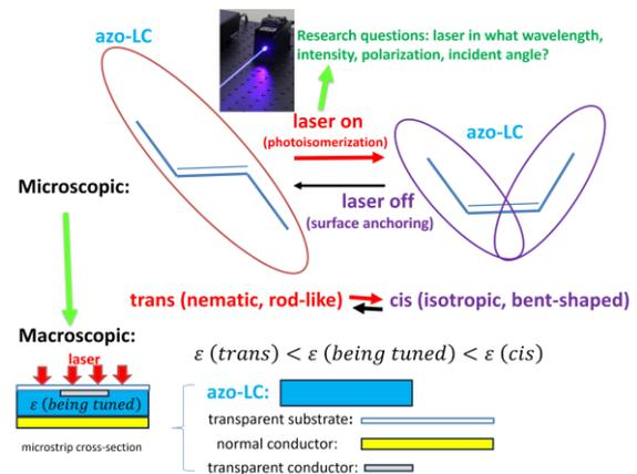
Fig. 1. Principle of trans-cis swap optically in azo-LCs for realizing MW tunable delay lines as we first developed [2].
