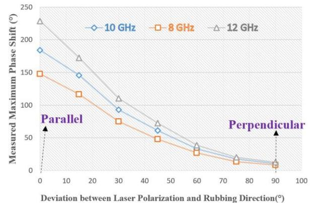
Fig. 3. Experimentally measured differential phase shift at X band with dependency on the deviation between laser beam polarization and rubbing direction (i.e., LC filling direction). Measurement results based on setup maintaining laser driving current of 3 A and incident angle of  $0^\circ$ .
