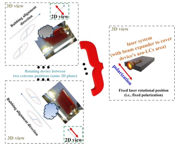
Fig. 2. Core experimental approach in polarization study (2D view represents fixed laser polarization relative to rubbing alignment direction that is rotating with device's rotation in the same 2D plane).
